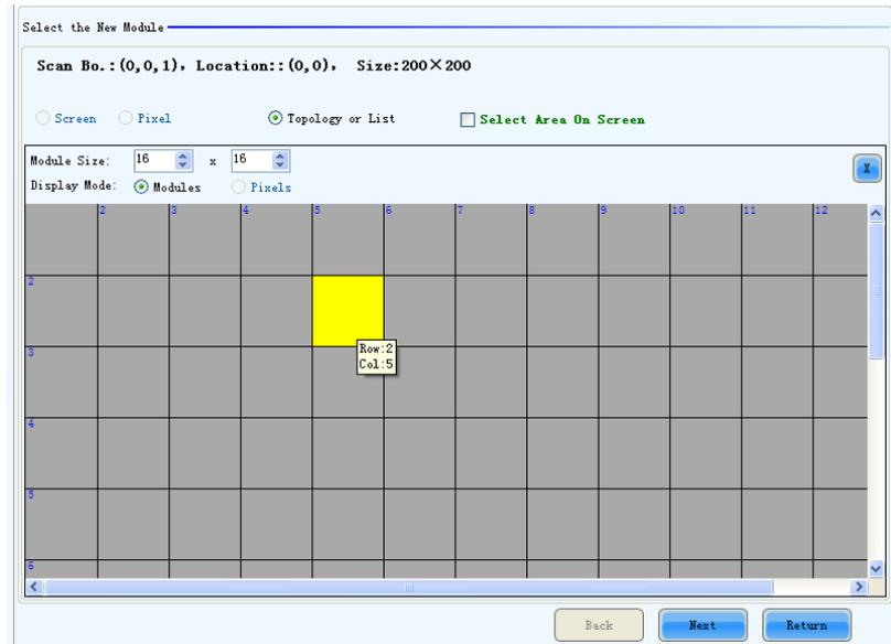
Fig. 7-75 Page for specifying the new module in the cabinet
