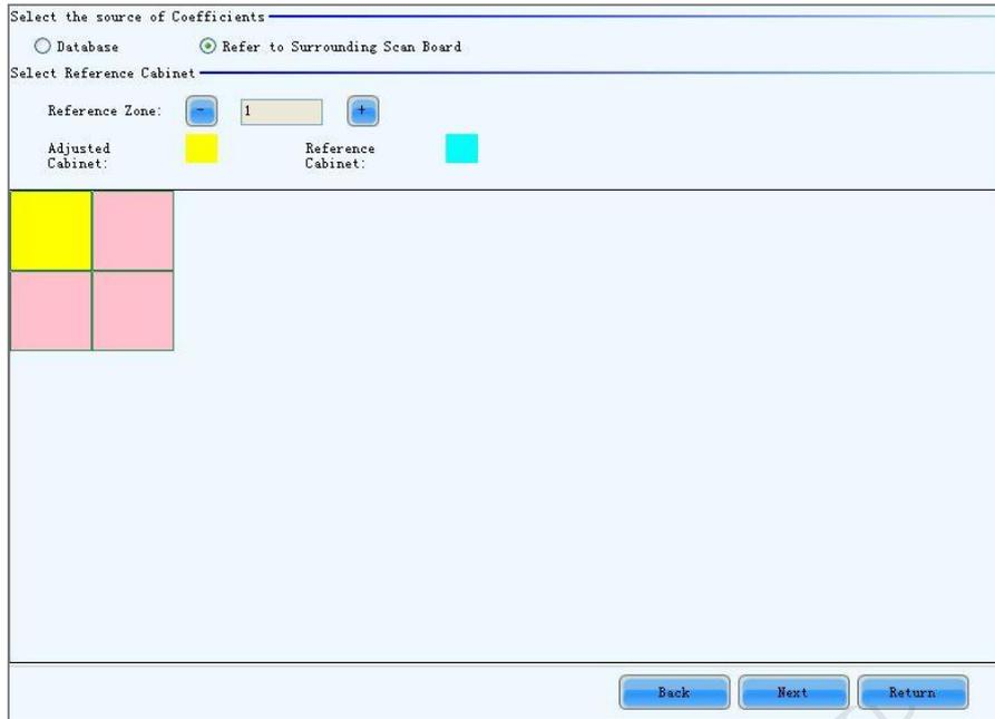
Fig. 7-70 Page for generating coefficients for the new scan board according to those of its surrounding scan boards
