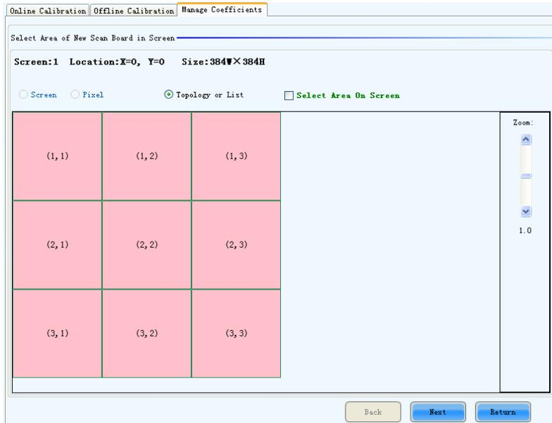
Fig. 7-68 Page for specifying the working area of the new scan board
