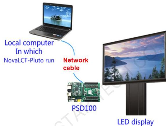
Fig. 5-1 Hardware Connection of NovaLCT-Pluto Configuration
