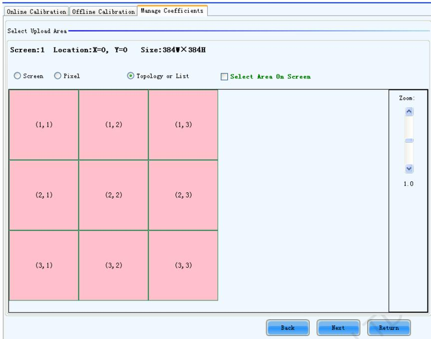
Fig. 7-63 Upload coefficients step 2- upload by Topology or list
